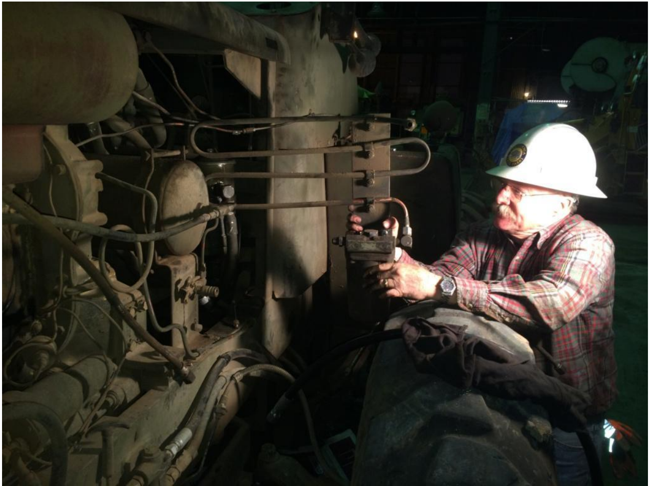
Mike H. re-assembling the air system on Big Green Machine
